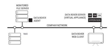
The Data Rover server is located within the customer's virtual infrastructure. Monitoring of storage resources (File Server or NAS) takes place via agents. The agent can be installed natively on Windows-based file servers or on a service machine to scan NAS devices.
